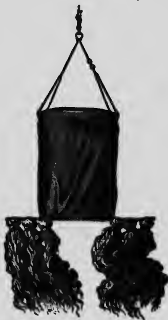
FIG. 156. — A deep-sea dredge. The iron lip of the sack scrapes shells, mud, etc., into it, and small animals are caught by the "tangles."
